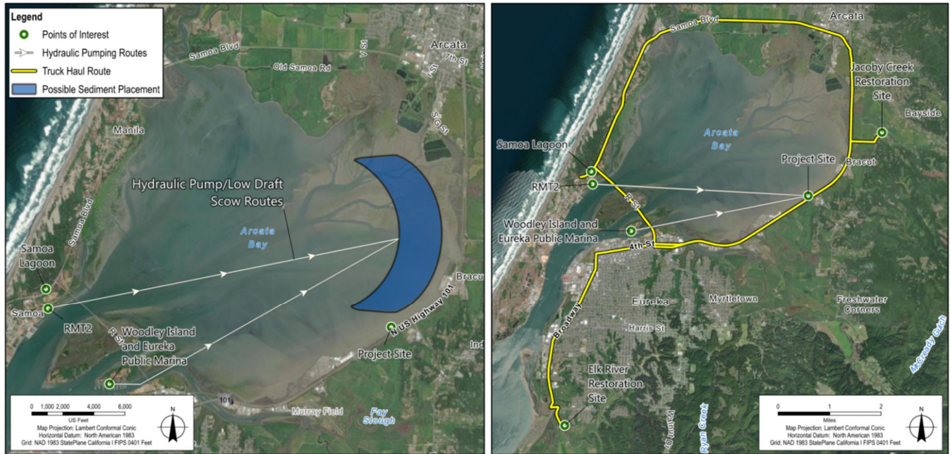
Figure 5 (left) and 6 (right). Possible routes for transporting sediment to the Project site are shown on the right. Indirect placement strategies are shown on the left.
