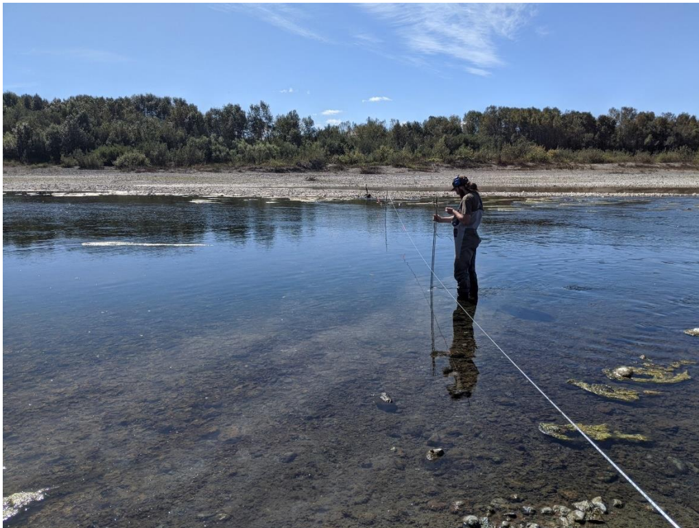
Figure 7. Streamflow measurement at QM-5
