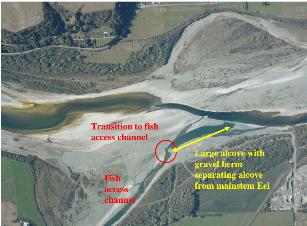
Figure 2. Alcove at confluence of Van Duzen River with Lower Eel (2004). Alcove transitions to fish access channel to aid Chinook salmon migration upstream into the Van Duzen River.
